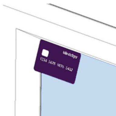
To correctly locate the bracket position, take a standard sized debit or credit card and hold it, sidewise, in the corner of the glass.
